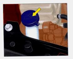
The anti-freeze contained in the coolant fluid allows it to maintain its performance at low temperatures, also giving it anti-corrosion properties and good performance at high temperatures. For this reason it is important to have the coolant fluid replaced every two years, at the start of the cold season, by a authorised dealer.
